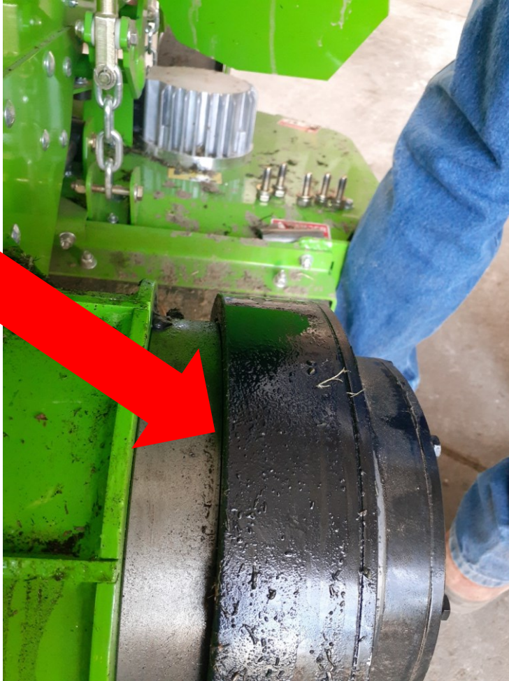
Leaking Hub Seal Location
